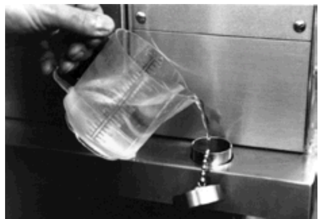
De-limer is poured through the port into the delimer reservoir.
