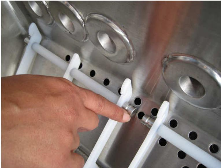
When you have placed all of the rear rib sets, begin placing front rib sets against the front wall of the sink. As with the rear rib sets, place the first front rib set against a corner, and leave a finger-size gap between it and the next front rib set.
