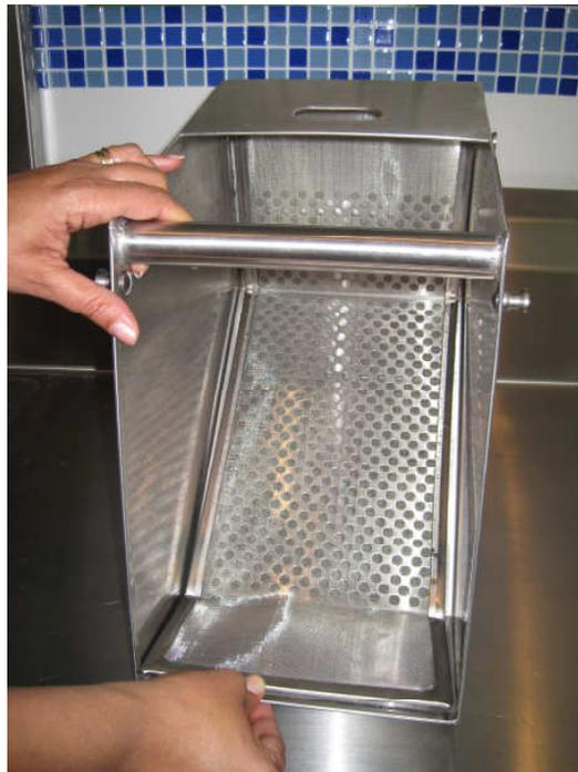
Allow a few minutes of collection time in each position. When finished, empty the contents of the filter into a suitable waste container, and wash out the filter and basket.
