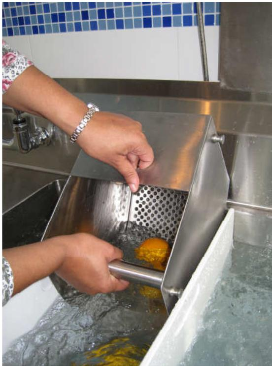
Rest the basket on the top edges of the partitions or the sink edges until all the produce is collected.
