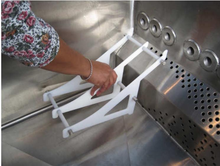
Place the other rear rib sets against the back wall of the sink leaving a finger-size gap between them.
