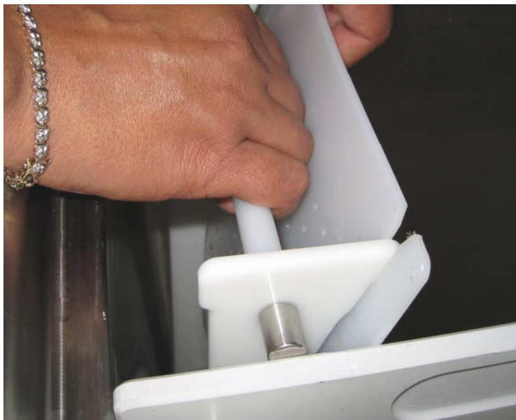
Repeat the process until all four flow guides are in place.
