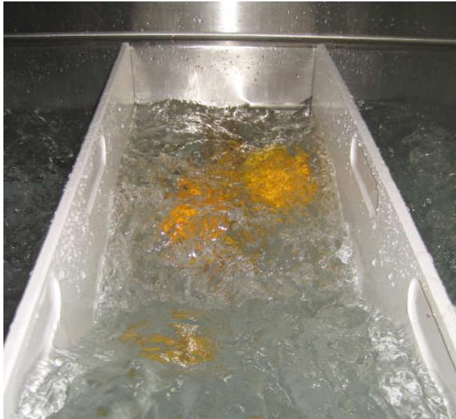
After the necessary time for soil removal and disinfection, the produce may be removed by inserting a collection basket. Holding the basket as shown, angle the basket so its leading edge is aligned with the flow in the sink.
